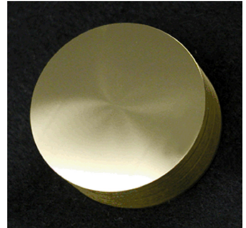
Light management array, 40 mm OD brass disk 620,000 lenses Lens pitch 45 \mu\text{m} , Lens form 250 \mu\text{m} R sphere.
